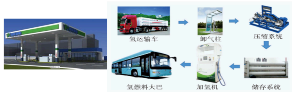
Hydrogen transport, refuelling and vehicle operation (project diagram)
