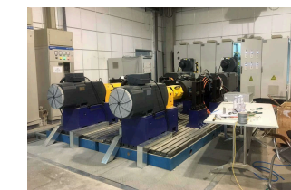
Multi-shaft powertrain test bench · Actual system
